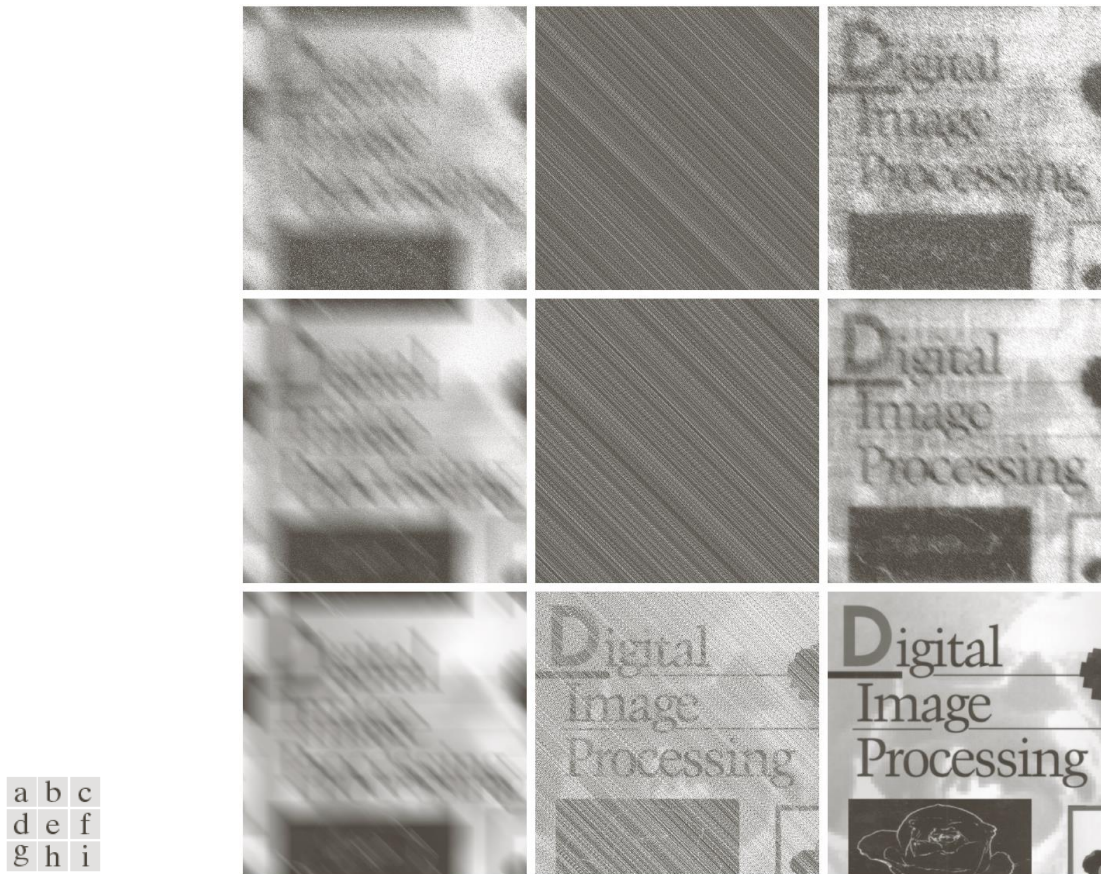
FIGURE 5.29 (a) 8-bit image corrupted by motion blur and additive noise. (b) Result of inverse filtering. (c) Result of Wiener filtering. (d)–(f) Same sequence, but with noise variance one order of magnitude less. (g)–(i) Same sequence, but noise variance reduced by five orders of magnitude from (a). Note in (h) how the deburred image is quite visible through a “curtain” of noise.
